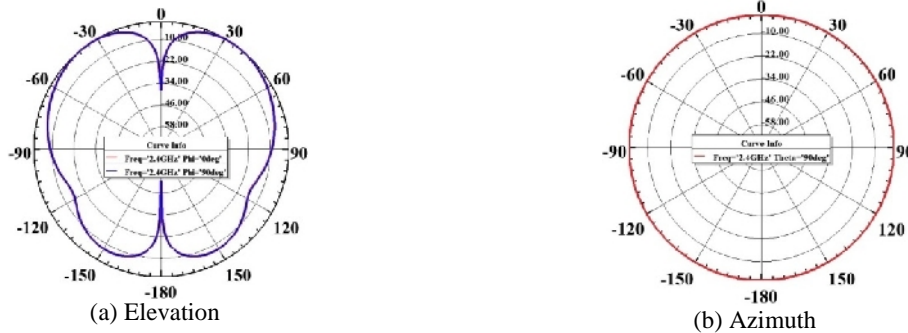
Fig. 9. 2D Radiation pattern for WLAN.
